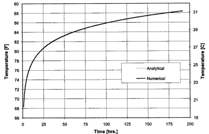
**Figure 8** Comparison of the numerical and analytical model temperature predictions. Test case #4. Pipe wall thickness approximated with 4 cells. Time step=3 minutes.
