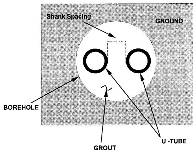
Figure 1 Cross-section of a typical borehole.
