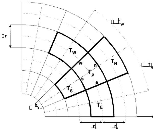
Figure 2 Notation of the finite control volumes.
