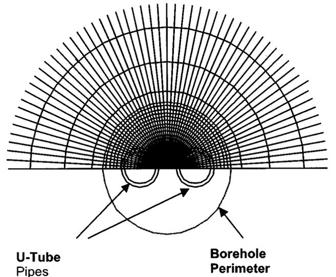
Figure 3 Example numerical grid near the borehole center.
