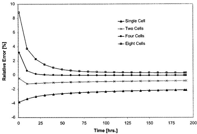
**Figure 5** Variation of the relative error of the calculated temperature with different grid resolution at the pipe wall (for test case #4 with 3-minute time steps).
