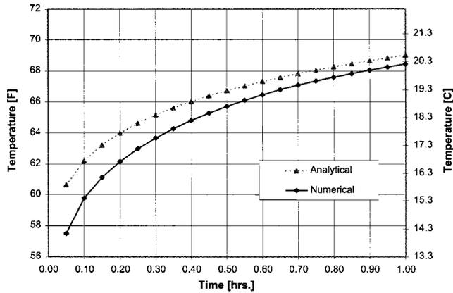
**Figure 9** Comparison of the numerical and analytical model temperature predictions over the first hour of simulation (test case #4).
