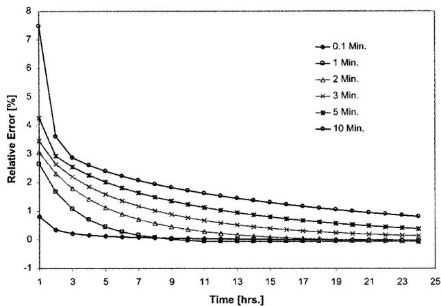
**Figure 6** Variation in the relative error of the calculated temperature with time step size (test case #4).
