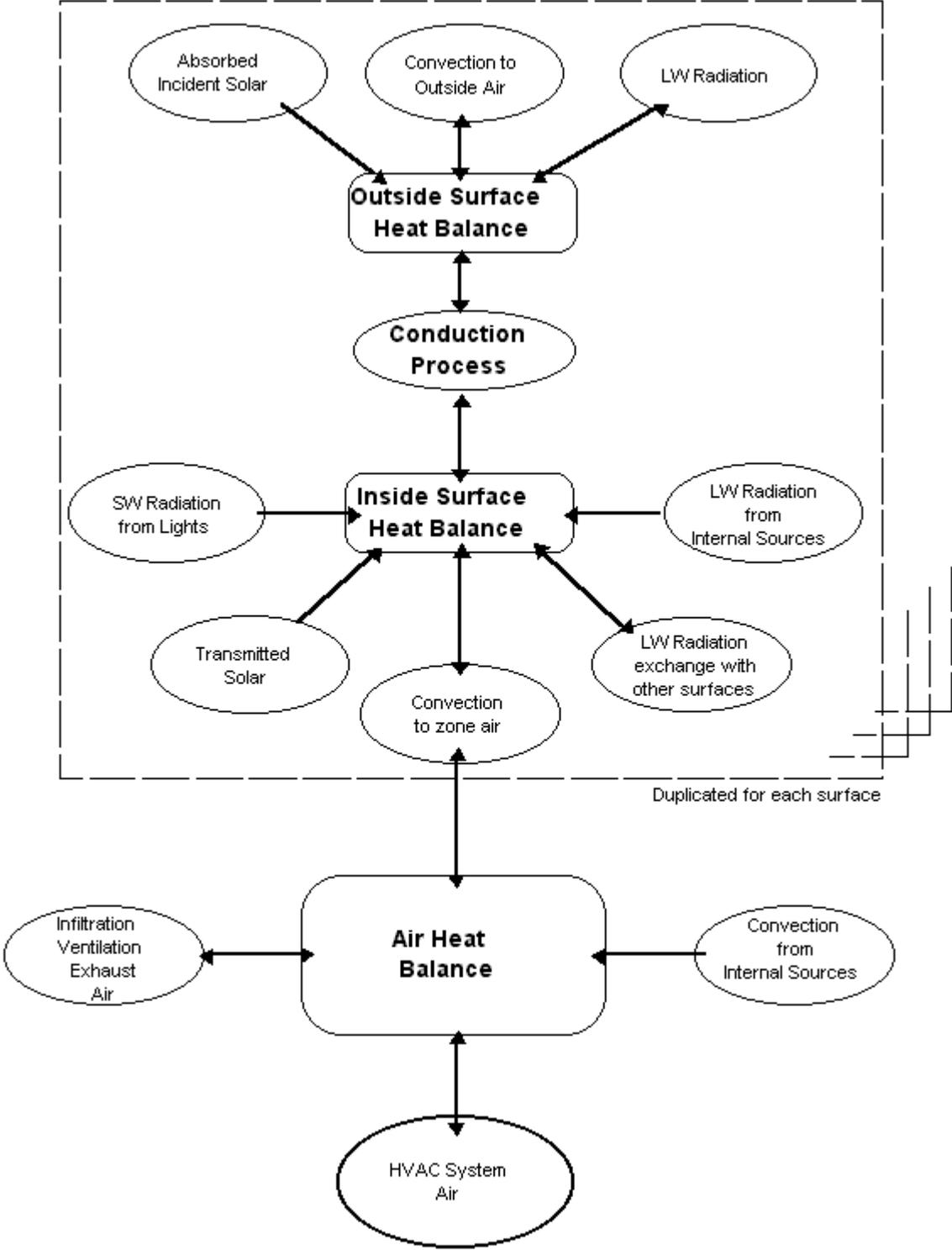
Figure 1. Schematic of the Energy Balance Processes in a Zone (Pedersen 1997).
