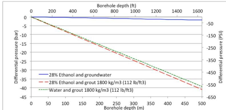
**Figure 2** Differential pressure in borehole with un-pressurized pipes.
