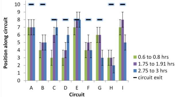
Figure 2: Circuit Two Phase Section End, for Different Time Periods, Frosting Test, EXV
