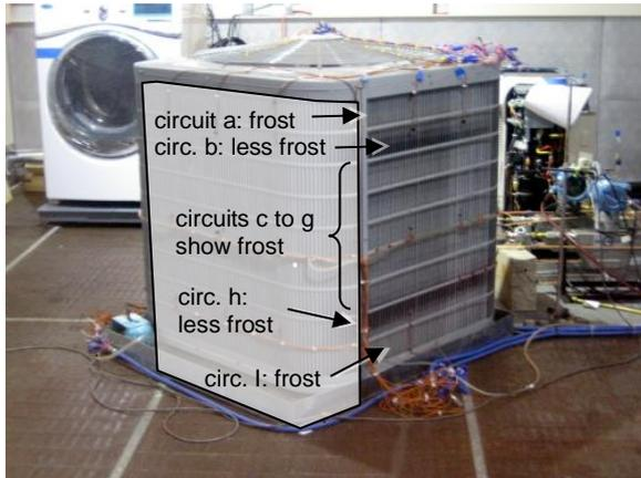
Figure 1: EXV Frosting Test, 0.47 hrs after Start
