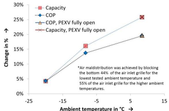
Figure 4: Performance Change after Implementing Hybrid Control, Blocked Coil Cases
