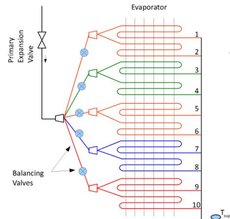
**Figure 6: Reduced Hybrid Control with Simplified Evaporator Layout**
