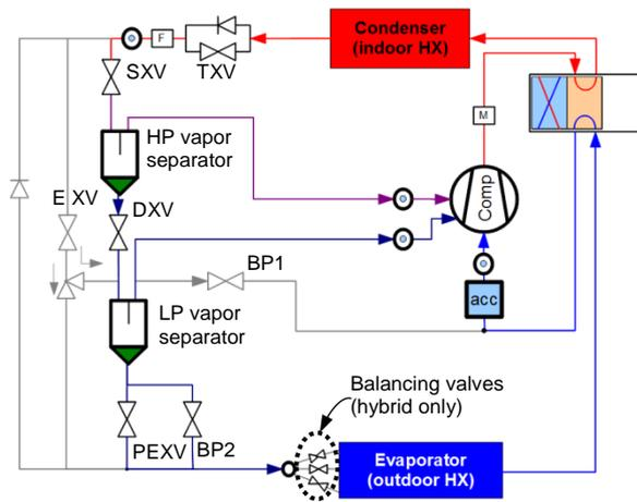
**Figure 5: Simplified System Schematic of Vapor Injected HP**
