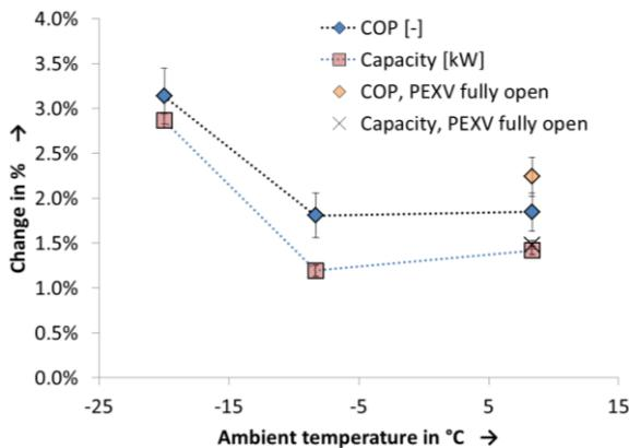
Figure 3: Performance Change after Implementing Hybrid Control, Clean Coil Cases
