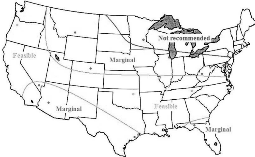
Figure 8 Preliminary feasibility of foundation heat exchangers for residential ground source heat pump systems.
