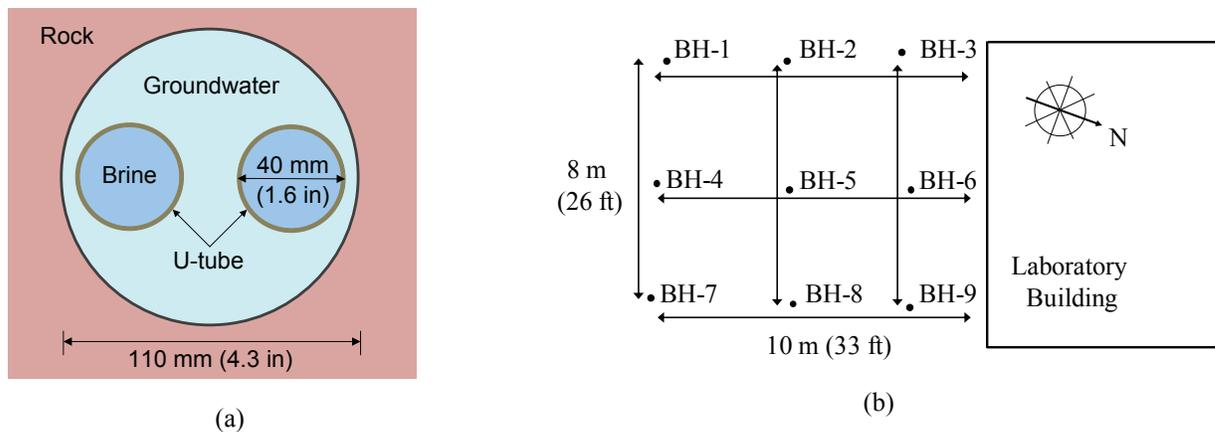
**Figure 1** Geometry and layout of the laboratory boreholes.
