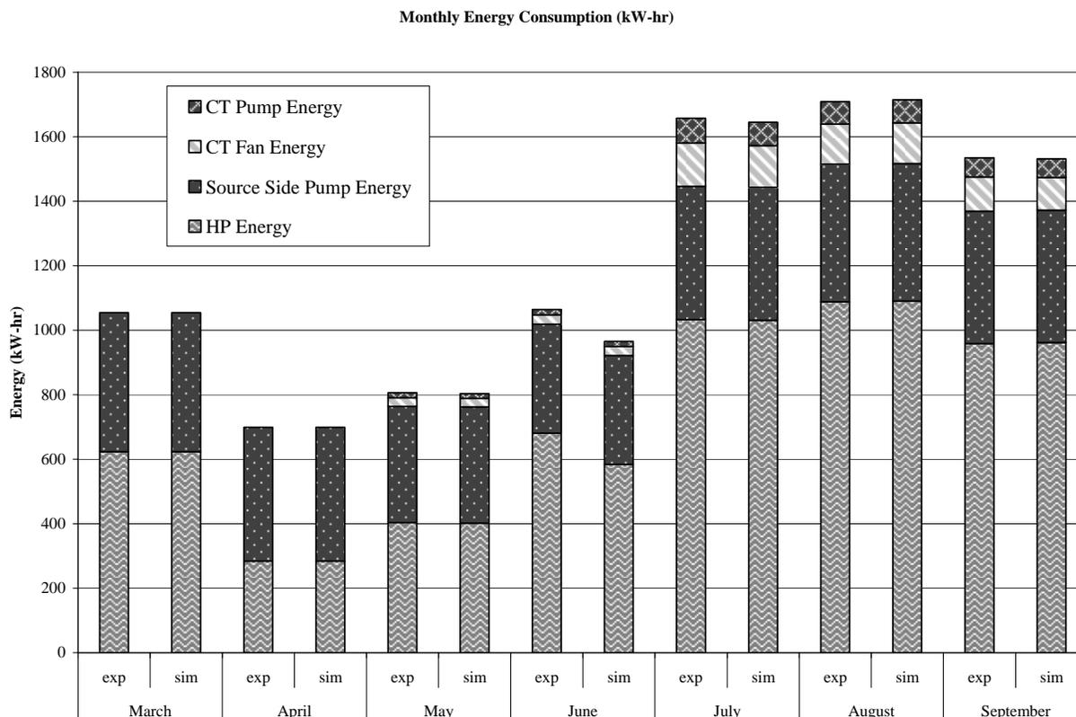
Figure 13. Experimental vs. simulated monthly energy consumption
