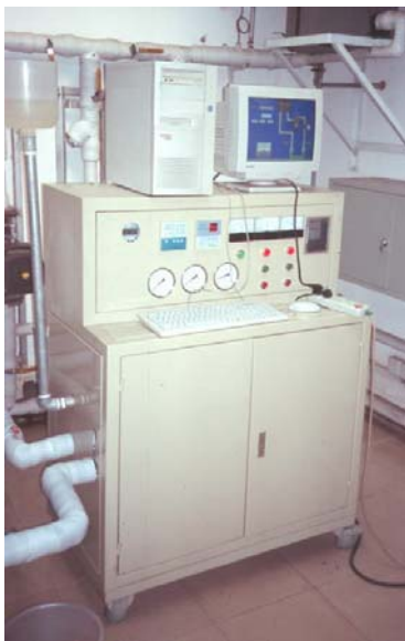
Fig. 7: Different thermal response test rigs, from above: Early rig from Landtechnik Weihestephan, rig built by UBeG for export to China, light rig built by hp system tech in South Korea, laboratory rig at Beijing University of Technology, China
