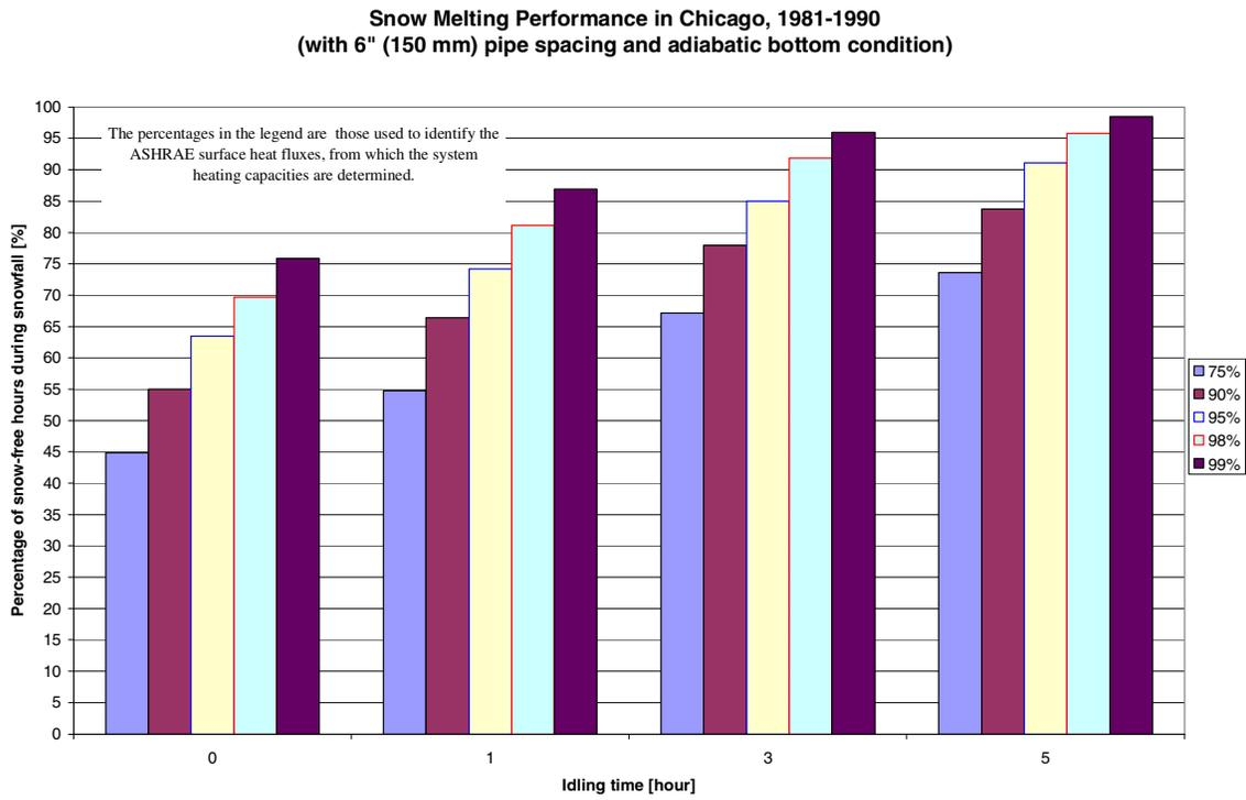
**FIGURE 2 Relationship among the idling time, heating capacity and snow melting performance at Chicago.**
