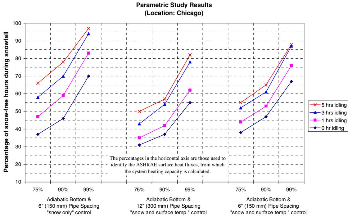
**FIGURE 7 Comparison of snow melting performance resulting from different combinations of control strategy and pipe spacing - Chicago.**
