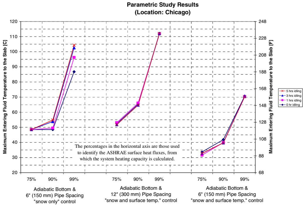
**FIGURE 8 Comparison of the maximum entering fluid temperature to the slab resulting from different combinations of control strategy and pipe spacing - Chicago.**
