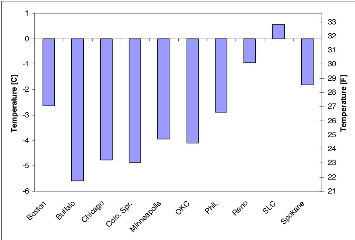
**FIGURE 4 Average coincident air dry-bulb temperature during snowfall.**
