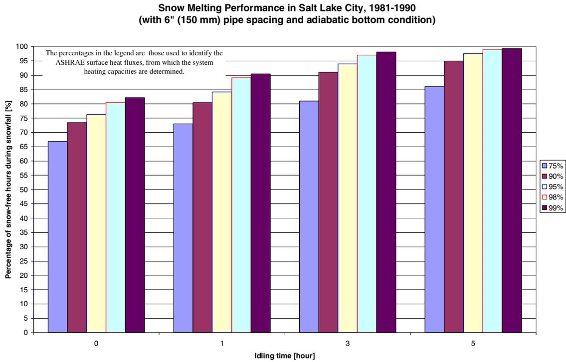
**FIGURE 3 Relationship among the idling time, heating capacity and snow melting performance at Salt Lake City.**
