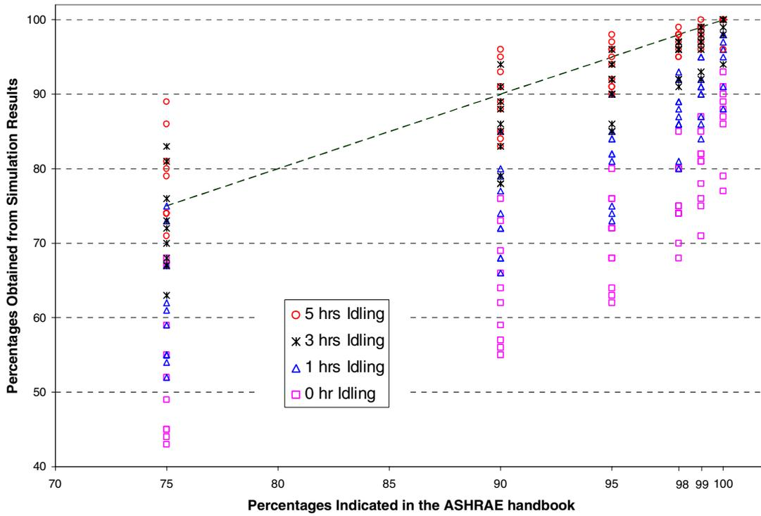
**FIGURE 1** Snow melting performances obtained from the simulation results of the first set of parametric study (Adiabatic bottom and edges with 6” (150 mm) pipe spacing).
