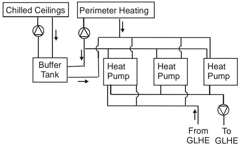
Figure 3: Conventional (Heating and Cooling) GSHP System
