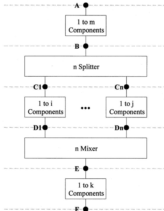
**Figure 2** Branch layout for individual HVAC subloops.
