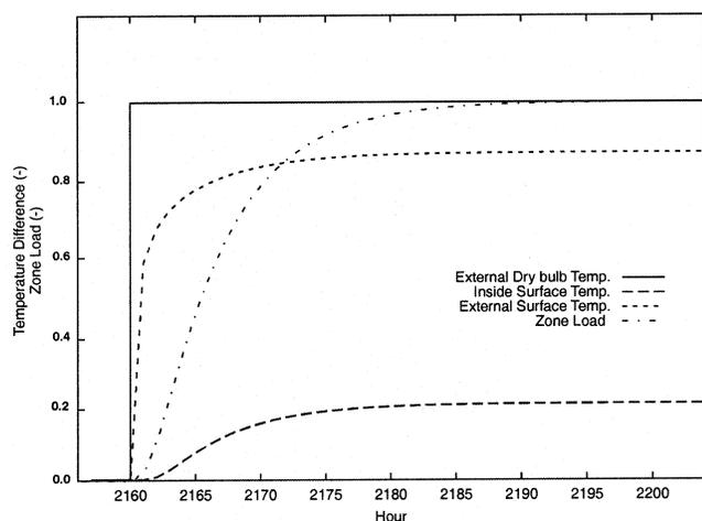
**Figure 3** The analytical solution for the transient conduction test TC2 for the 48 hours around the first step change in outside dry-bulb temperature. The temperature and zone loads are nondimensionalized.
