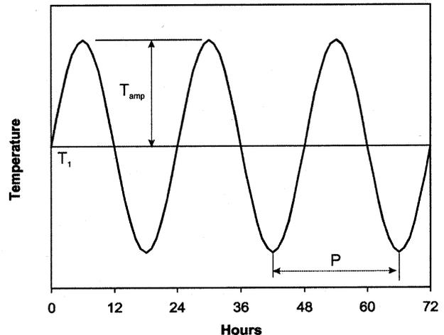
**Figure 1** Driving external dry-bulb temperature profiles used in the transient conduction tests: (a) a stepped profile used in tests TC1 and TC2, (b) the sinusoidal profile used in test TC3.
