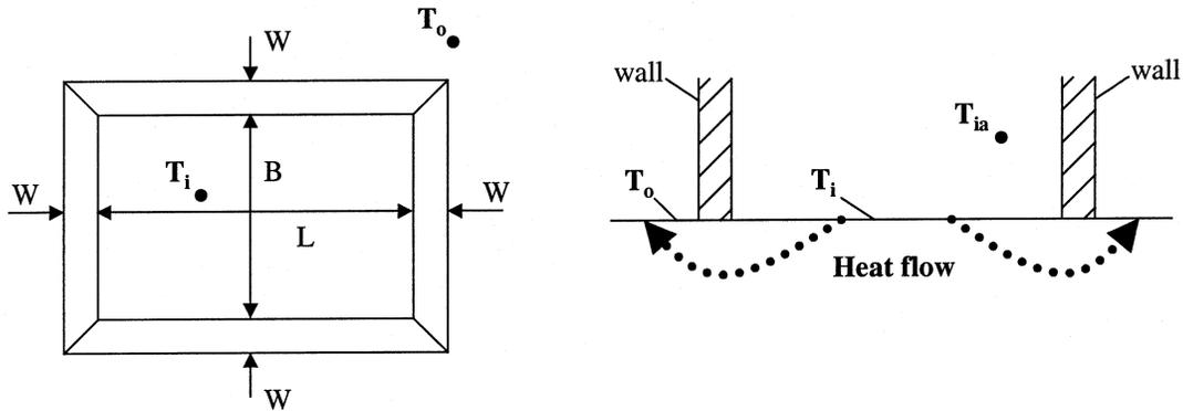
**Figure 6** A plan view (left) and section view (right) of the ground and wall geometry.  $T_{ia}$  is the inside air temperature,  $T_i$  is surface temperature of the floor, and  $T_o$  is temperature of the outside ground.
