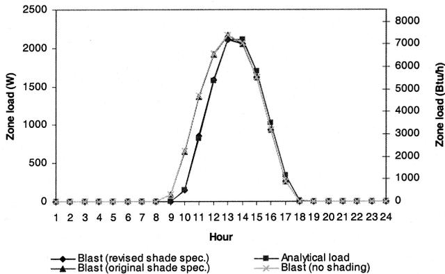
**Figure 9** Comparison of zone loads with alternative shade specifications: right-side wing on a south-facing window.
