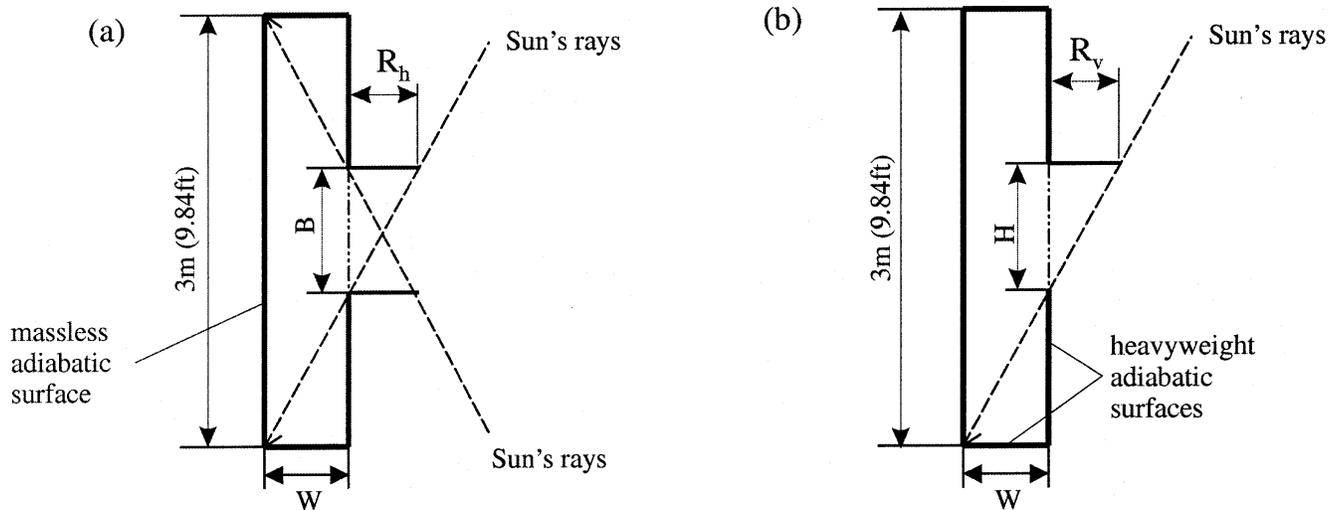
**Figure 4** Zone geometry of the internal solar distribution test: (a) plan view showing two vertical fins, (b) vertical view showing horizontal fin at the top of the window. The dimensions  $W$ ,  $R_v$ , and  $R_h$  are 0.5 m (1.64 ft), and the dimensions  $H$  and  $B$  are 1.0 m (3.28 ft).
