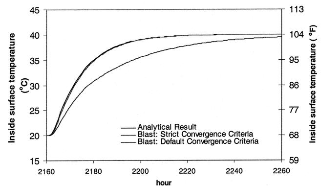
**Figure 8** Inside surface temperature response for test TCI using different convergence criteria.
