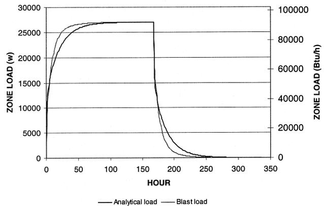
**Figure 7** Analytically calculated zone loads and those predicted by the BLAST program for the internal heat gain test.
