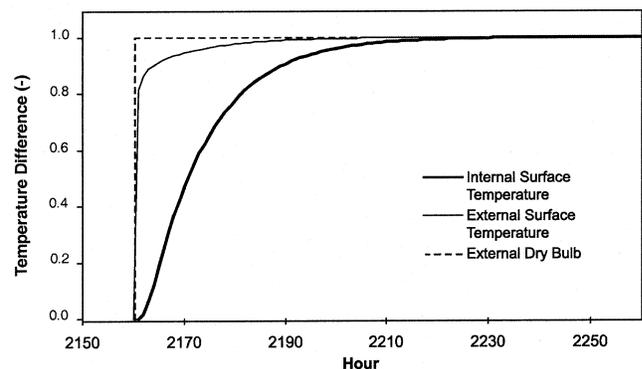
**Figure 2** The analytical response in surface temperatures in the transient conduction test case TC1. The temperatures are nondimensionalized.
