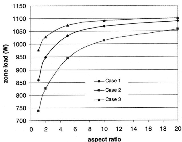
**Figure 5** Zone load variation with zone aspect ratio and different surface emissivities. The emissivities are: Case 1, external surface 0.9, opposite surface 0.1, other surfaces 0.3; Case 2, external surface 0.9, all other surfaces 0.1; Case 3, all surfaces 0.9.
