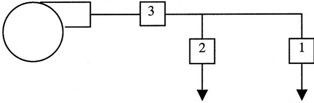
Figure 1 Hypothetical three-section duct system.
