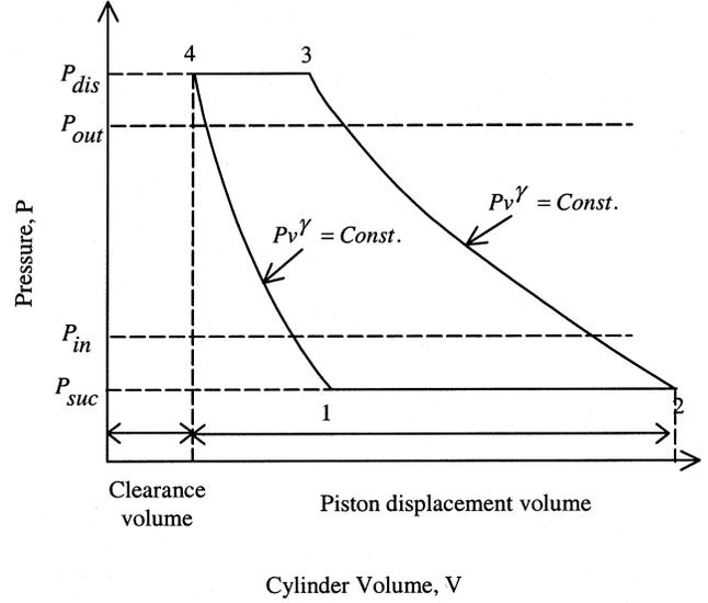
**Figure 2** Schematic indicator diagram for a reciprocating compressor.
