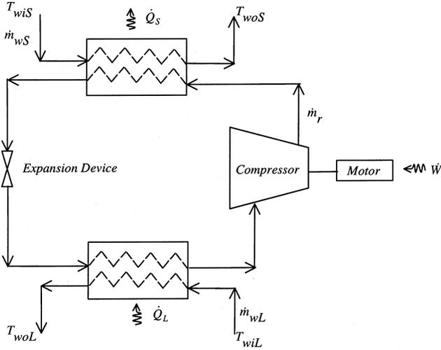
**Figure 1** Basic heat pump configuration.
