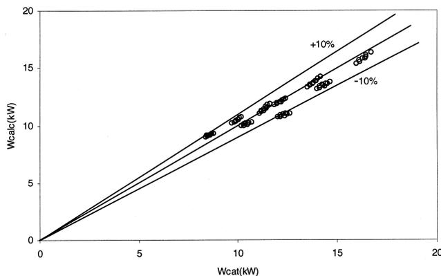
Figure 7 Calculated power versus catalog power (heat pump B).
