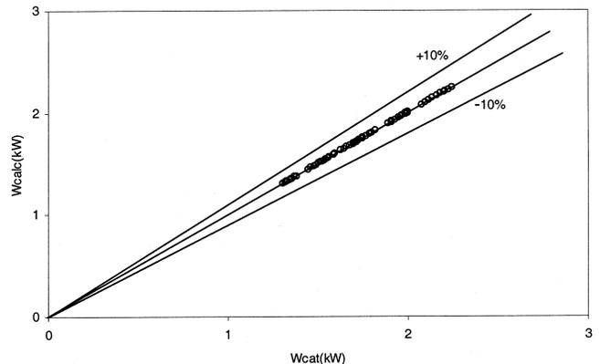
Figure 9 Calculated power versus catalog power (heat pump A).
