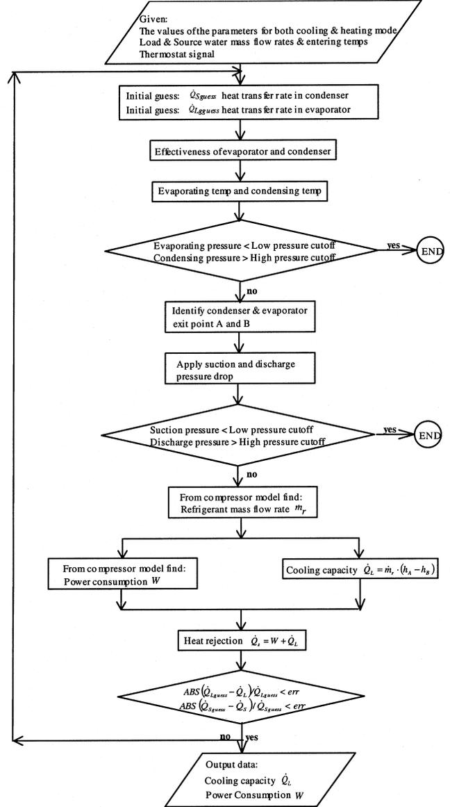
Figure 5 Flow diagram for model implementation computer program.
