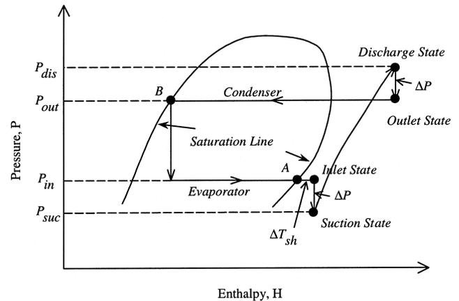
Figure 3 Pressure-enthalpy diagram for the refrigeration cycle.
