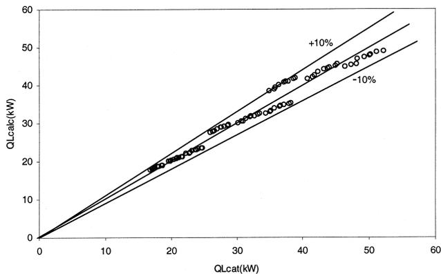
Figure 6 Calculated cooling capacity versus catalog cooling capacity (heat pump B).
