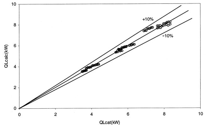
Figure 8 Calculated heating capacity versus catalog heating capacity (heat pump A).
