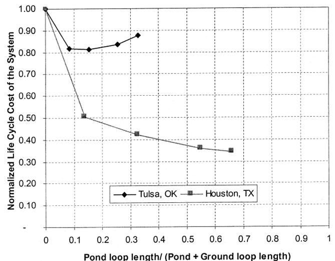
**Figure 7** Normalized life-cycle cost of the GSHP system vs. the ratio of pond loop length to total loop length for Houston, Tex., and Tulsa, Okla., climatic conditions.
