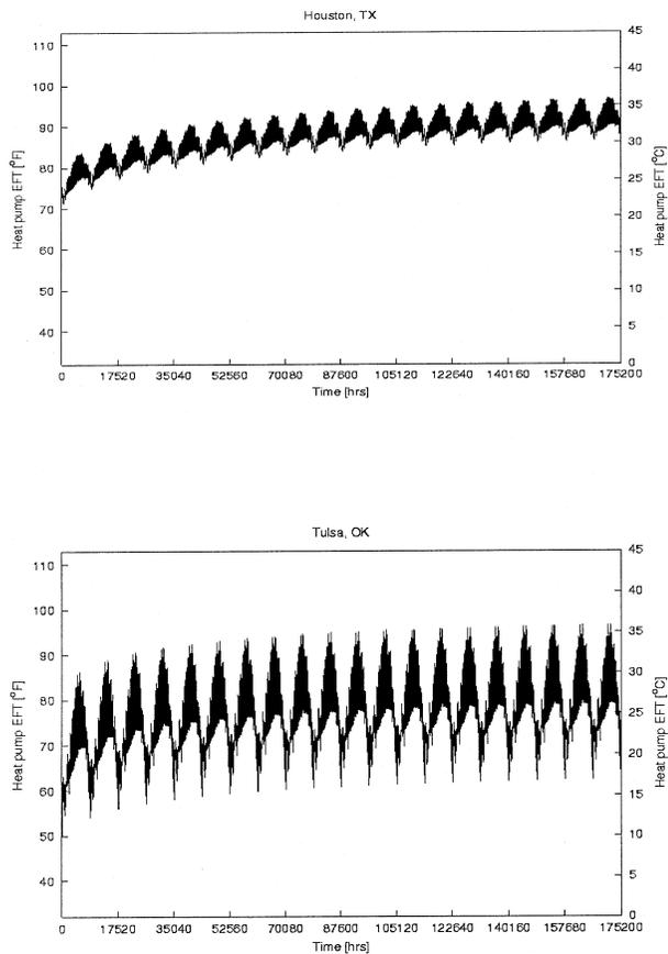
**Figure 3** Hourly entering fluid temperatures to the heat pump for Houston, Tex., and Tulsa, Okla., climatic conditions—ease 1 (base case).
