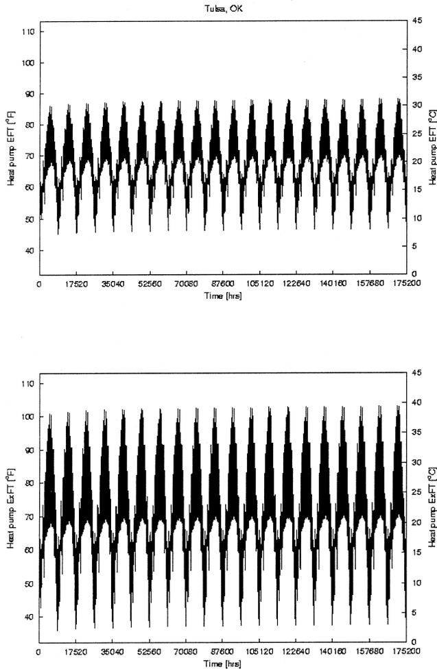
**Figure 4** Hourly heat pump entering fluid (EFT) and exiting fluid (ExFT) temperatures for Tulsa, Okla., climatic conditions-ease 3.
