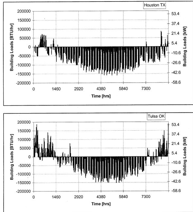
**Figure 1** Annual building loads for climatic conditions typical of Houston, Tex., and Tulsa, Okla. (cooling loads are negative and heating loads are positive).
