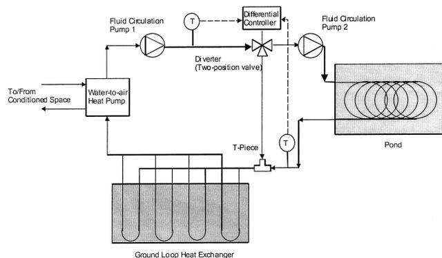
**Figure 2** Schematic diagram of the hybrid system component configuration.
