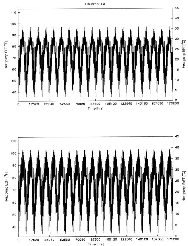
**Figure 5** Hourly heat pump entering fluid (EFT) and exiting fluid (ExFT) temperatures to the heat pump for typical Houston, Tex., climatic conditions; 20-year simulation-ease 5.
