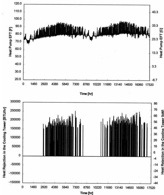
**Figure 6** Hourly entering fluid temperatures to the heat pump and heat rejection in the cooling tower for typical Houston, Texas, climatic conditions—two-year simulation, case 3a.
