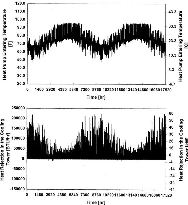
**Figure 9** Hourly heat pump entering fluid temperature and heat rejection in the cooling tower for Houston, Texas typical weather conditions and using control strategy 5a for the first two years of simulation.
