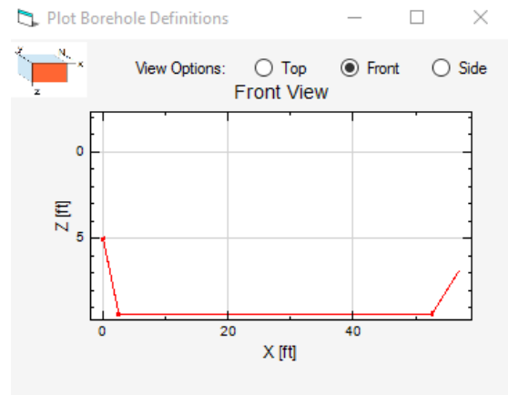
A horizontally-drilled borehole.
