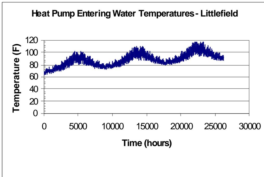
**Figure 1.** Increase in the heat pump entering water temperature without supplemental heat rejecters.
