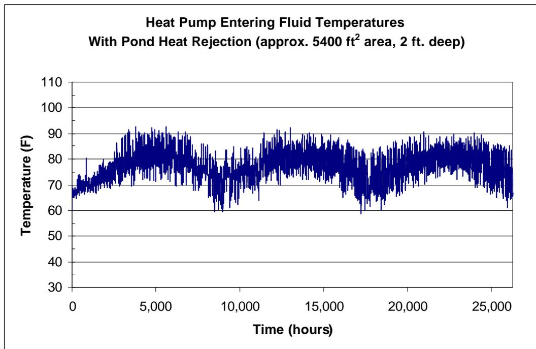
**Figure 3.** The heat pump entering water temperature with the pond model.
