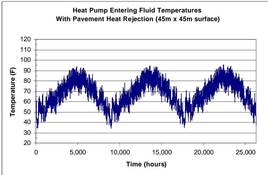
**Figure 2.** The heat pump entering water temperature with the pavement-heating model.
