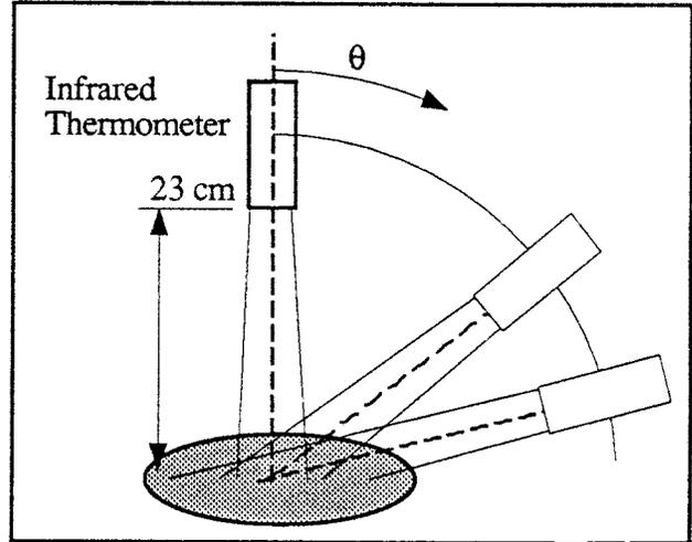
Figure 6 Experimental setup for angular emissivity experiments.
