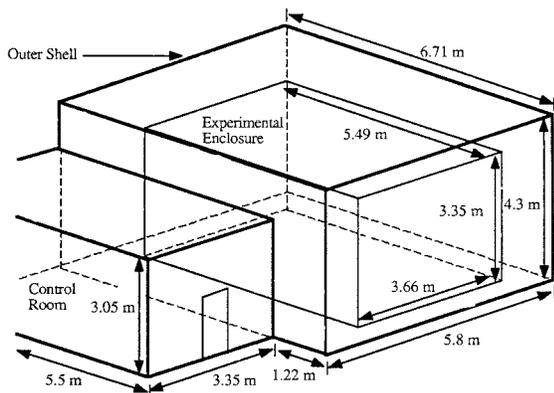
Figure 3 Schematic of experimental facility (Fisher 1989).
