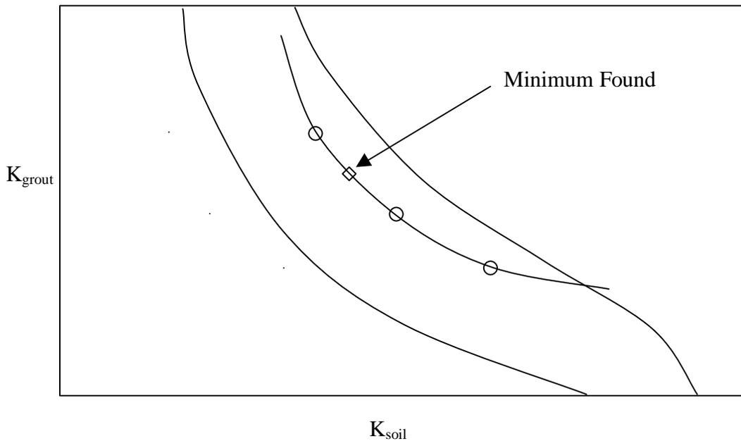
Figure 3-7. Quadratic Curve fitting in a valley
