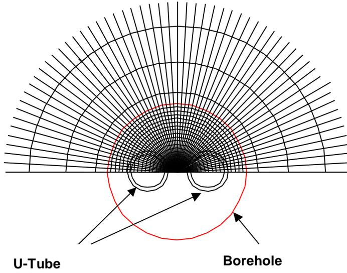
Figure 1-2. Domain for numerical model
