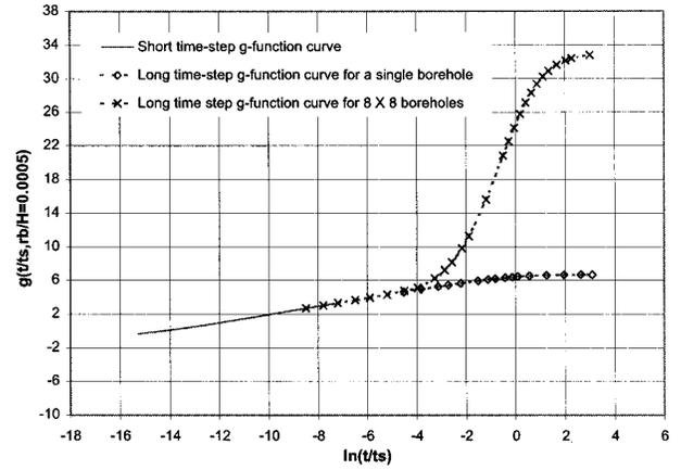
Figure 4 Short time-step  $g$  function curve as an extension of the long time-step  $g$  functions plotted for a single borehole and an 8×8 borehole field.
