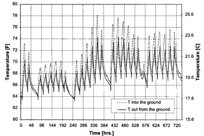
**Figure 12** Hourly input and output temperatures to the ground during the month of January for the example building in Tulsa, Oklahoma.
