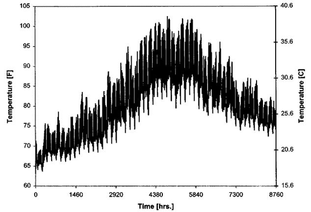
**Figure 11** Hourly average borehole temperature profile for the example building in Tulsa, Oklahoma as a result of an annual simulation with TRNSYS.
