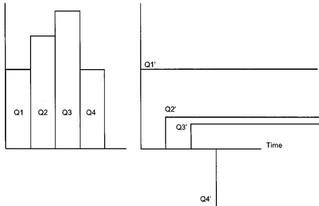
**Figure 1** Superposition of piecewise linear step heat inputs in time. The step heat inputs  $Q_2$ ,  $Q_3$ , and  $Q_4$  are superimposed in time on to the basic heat pulse  $Q_1$ .
