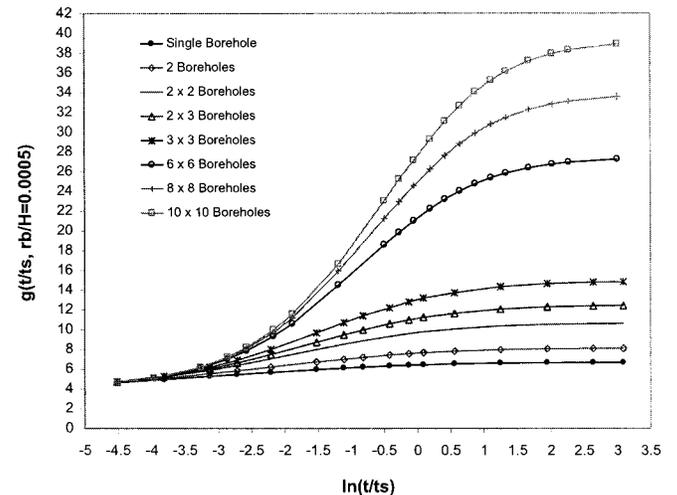
**Figure 2** Temperature response factors ( $g$  functions) for various multiple borehole configurations compared to the temperature response curve for a single borehole.
