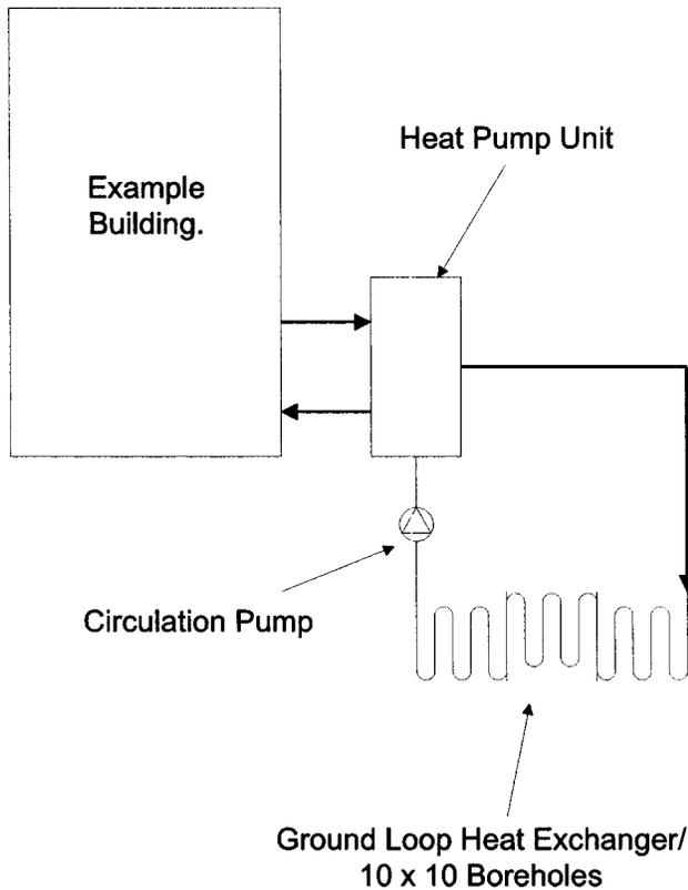
**Figure 10** A very simple schematic configuration of the example building setup.
