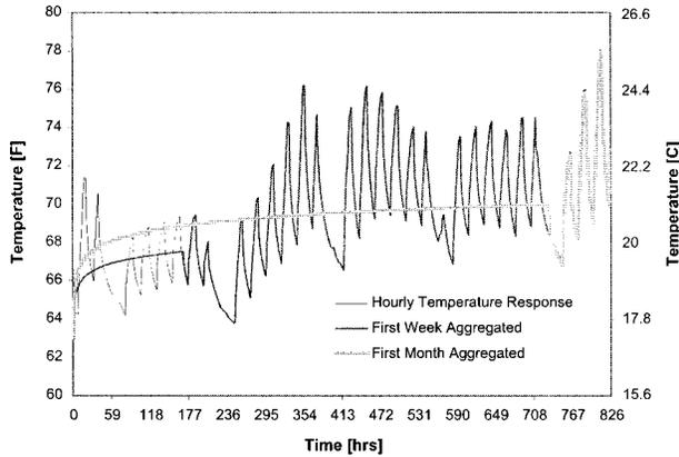
**Figure 5** Comparison of temperature responses based on hourly loads with temperature responses obtained through load aggregation for first week average and first month average loads for a typical case.
