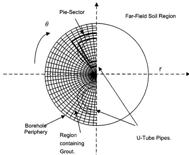
**Figure 3** Simplified representation of the borehole region on the numerical model domain using the pie-sector approximation for the U-tube pipes.
