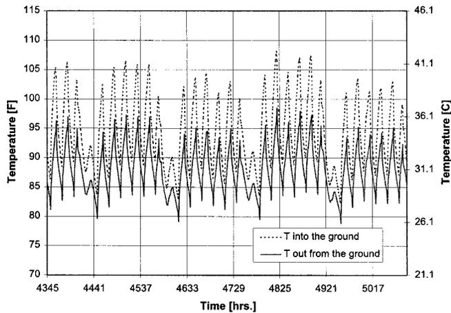
**Figure 13** Hourly input and output temperatures to the ground during the month of July for the example building in Tulsa, Oklahoma.
