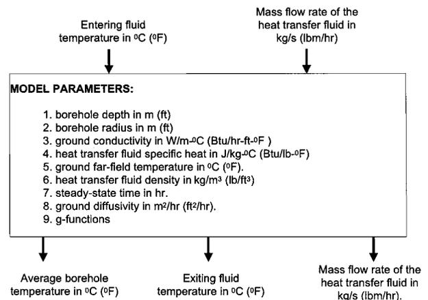
Figure 8 TRNSYS short time-step component model configuration.
