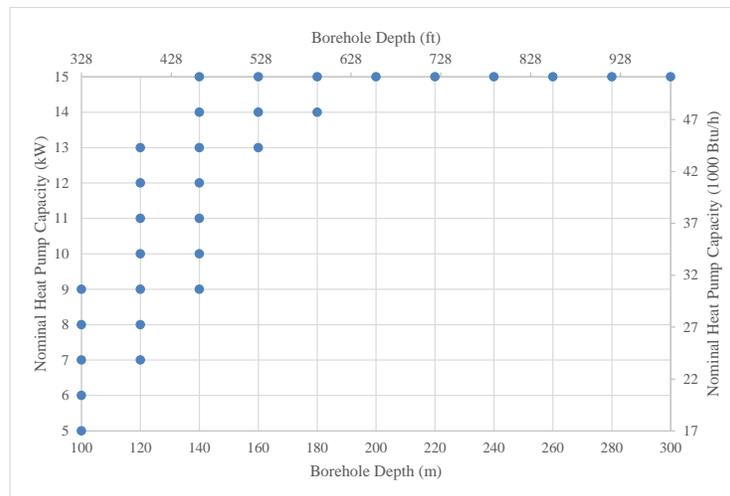
**Figure 5** Heat Pump Capacity – Borehole Depth Combinations Corresponding to Pareto Front
