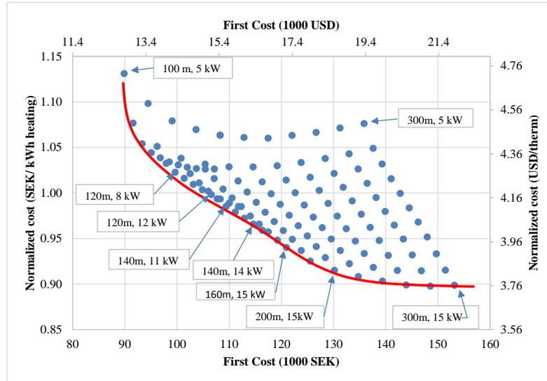
**Figure 4** Normalized Life Cycle Cost vs. First Cost with Pareto Front Marked
