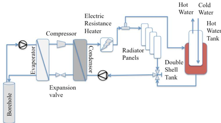
**Figure 2** Typical Swedish Ground Source Heat Pump with Integrated Hot Water Storage Tank and Electric Resistance Heater.
