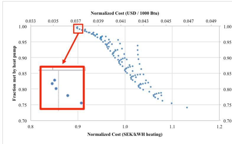
**Figure 3** Fraction of heating load met by heat pump vs. normalized life cycle cost
