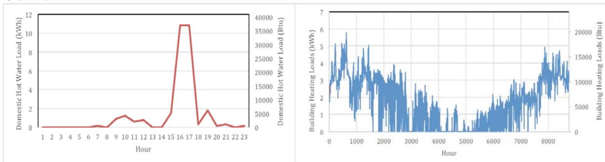
**Figure 1** a) Daily Domestic Hot Water Load b) Annual Building Heating Loads
