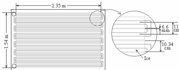
Figure 6. A branch of ice storage with horizontal tubes in fully charged condition.
