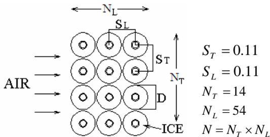
Figure 7. Tube bank configuration.
