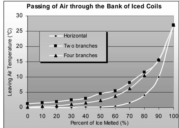
Figure 8. Air leaving temperature passing through the bank of iced tubes. Air entering temperature is 27°C (80°F)
