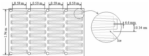
Figure 10. Bank of coils when four branches are used
