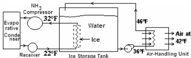
Figure 1. Schematic diagram of components and temperatures in a storage system with cold air distribution
