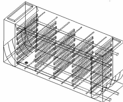
Figure 2. External melt ice storage tank with a special inlet and outlet section to guide air flow in discharge time.
