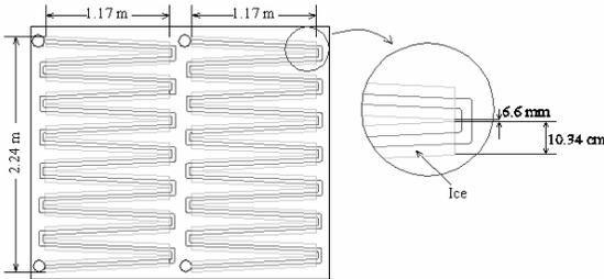
Figure 9. Bank of coils when two branches are used
