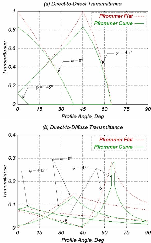
Figure 7 Effect of Slat Curvature (for Curved Slat with R/W Ratio of 1.0 and Slat Reflectance of 0.5): (a) Direct-to-Direct Transmittance, (b) Direct-to-Diffuse Transmittance
