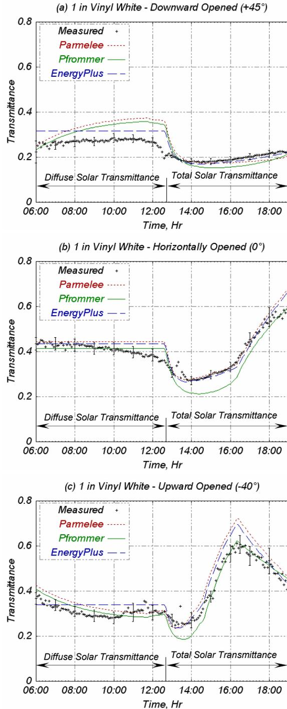
Figure 8 Experimental Comparison Results: a) Downward Opened (+45°), b) Horizontally Opened (0°), and c) Upward Opened (-40°).
