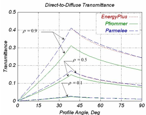
Figure 3 Effect of Slat Reflectance on Direct-to-Diffuse Transmittance (for Flat Slat with Zero Thickness, and Slat Angle of 0°)
