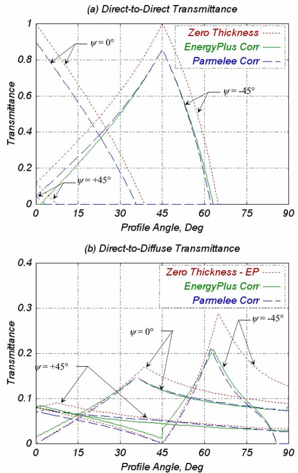
Figure 6 Effect of Slat Thickness (for Flat Slat with T/S Ratio of 0.1 and Slat Reflectance of 0.5): (a) Direct-to-Direct Transmittance, (b) Direct-to-Diffuse Transmittance
