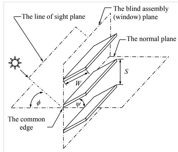
Figure 1 Profile Angle and Slat Geometry ( $\phi$  = the profile angle,  $\psi$  = the slat angle,  $S$  = the slat spacing,  $W$  = the slat width)
