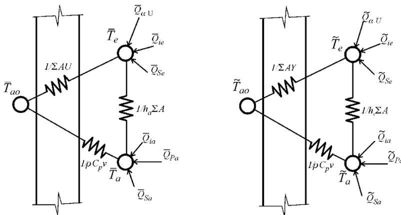
**Figure 4. CIBSE Admittance cooling load calculation method represented as a nodal network. Different networks are used for the steady state (left) and fluctuating components (right) of the heat gains and loads.**
