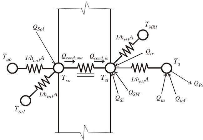
**Figure 2. ASHRAE Heat Balance cooling load calculation method represented as nodal network A single wall is shown with the outside surface on the left**
