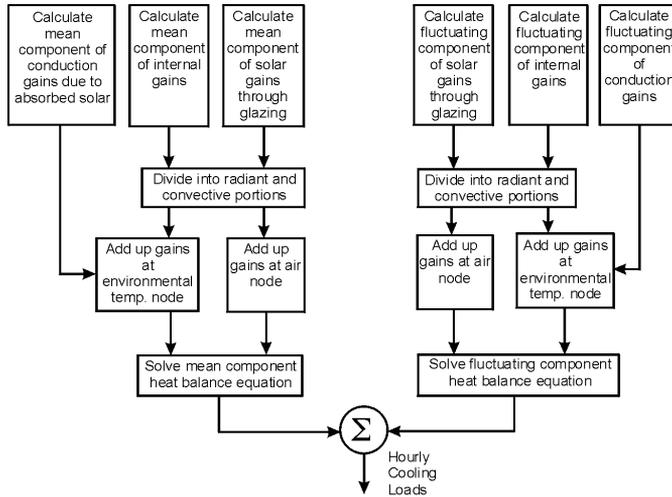
**Figure 7. CIBSE Admittance cooling load calculation method represented as a flow diagram**
