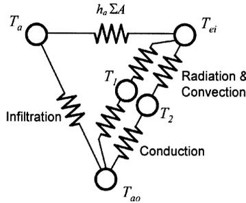
**Figure A3. Inclusion of loss conductances: Infiltration and conduction**
