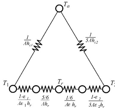
**Figure A4. Figure 1 modified so as to derive a valid global temperature (Links are shown as resistances with units of K/W)**
