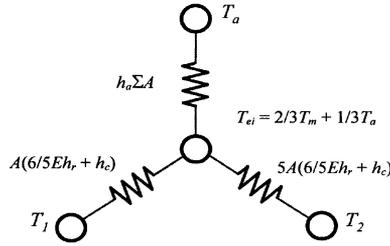
**Figure A2. Merging of radiant and convective exchanges and environmental temperature**
