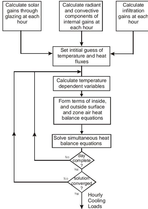
**Figure 5. ASHRAE Heat Balance cooling load calculation method represented as a flow diagram**
