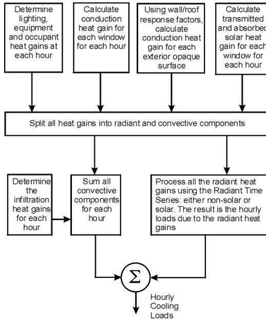
**Figure 6. Radiant Time Series cooling load calculation method represented as flow diagram**
