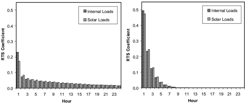
Figure 8. RTS coefficients for typical heavyweight (left) and lightweight (right) zone
