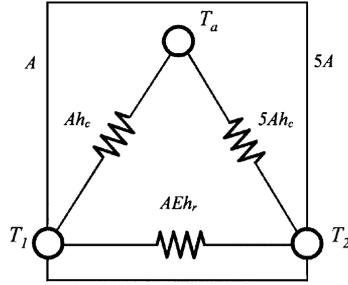
**Figure A1. CIBSE Guide enclosure model (links are conductances with units of W/K)**
