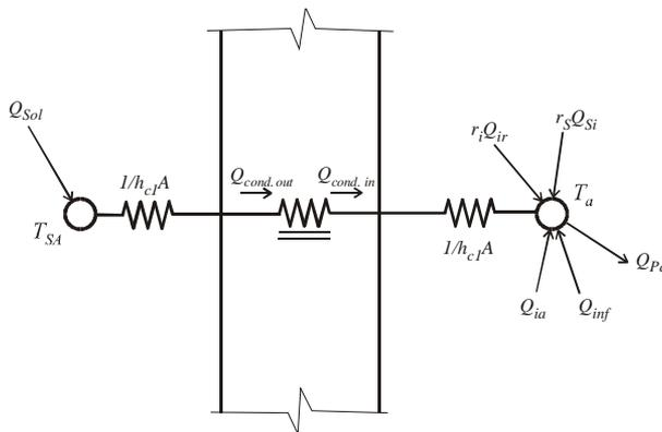
**Figure 3. Radiant Time Series cooling load calculation method represented as a nodal network. A single wall is shown with the outside surface on the left.**
