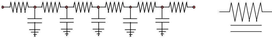
**Figure 1. Approximation of wall with thermal mass as series of lumped capacitances (left) and its representation (right) in nodal network diagrams of Heat Balance and RTS calculation methods**
